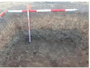
Plate 6.16 TP 5, north section, showing the stratified layers of compact fill
