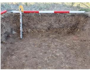
Plate 6.14 TP 3, north section, showing compact shale and clay fill with thin gravelly topsoil
