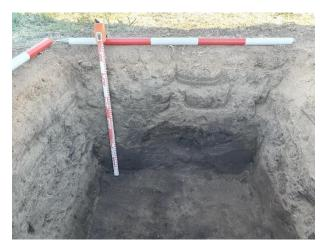
TP6 north section, showing a silty clay B2 horizon, with increasing compaction at depth **Plate 6.18**
