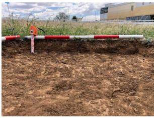
Plate 6.12 TP 2, north section, showing compact clay base and thin gravelly topsoil
